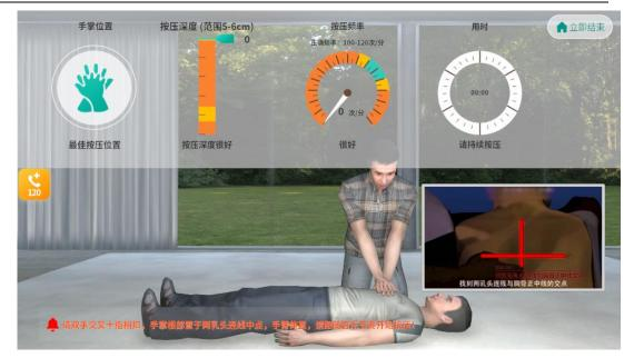
The simulator will record all the key operations in the CPR procedure including, pressing depth, press frequency, chest spring back, time use, etc. The record will shows on the screen in real time. The trainer can the adjust operations immediately with the tips appears in real time. The training efficiency is very high.
